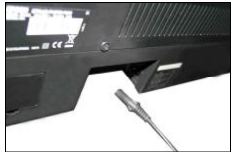
pulling out the power line of the printer and move the cartridge bar to the cartridge-changing side.
