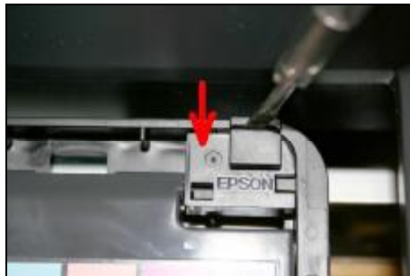
Inserting the above screwdriver into the the gap and prize it slowly as picture shown. Don't prize it overexert.
