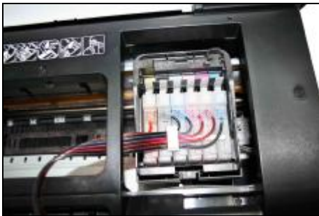
Put in the cartridge of CISS according to the color mark and lock the cartridge.
