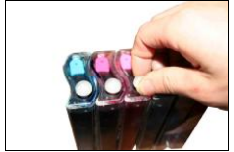
Place an air filter into each air hole. (6pcs for 6 air holes total)
