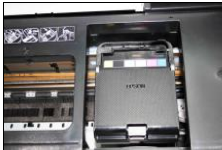
pulling out the power line of the printer and move the cartridge bar to the cartridge-changing side.
