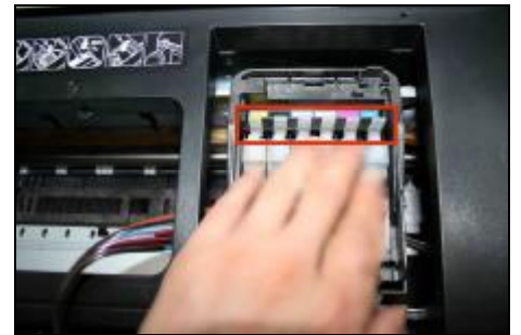
A sound "Da" will be heard when the clip Has Locked the cartridge completely
