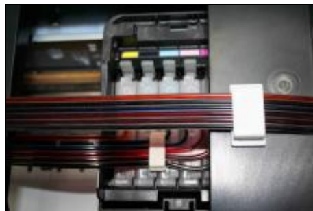
Place the tubes orderly into the small clips And clips them well
