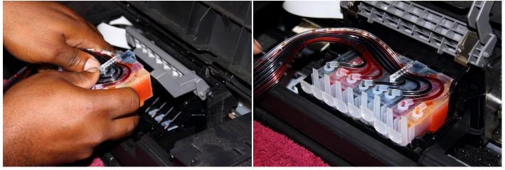
You can attach one clip in the center of the link, then arrange the tube, please make sure the tubes are not twisted, you need to leave the lid open after you install the ciss
