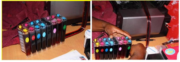
Open the small plugs (air hole) on the top of ink reservoir
